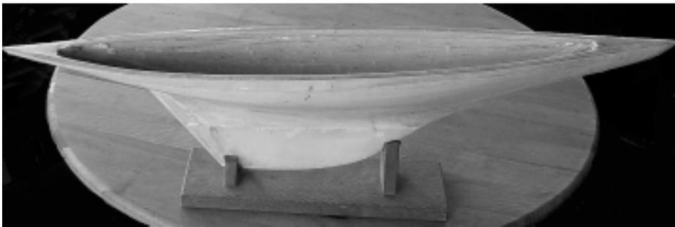
The final hull, faired, glassed and with the sheer cut. All the mechanical details, etc., are the same as for *Yankee III*.
