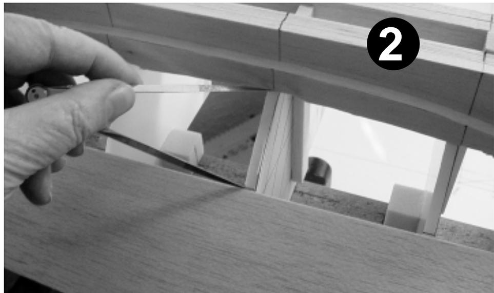
2. Lay a balsa board that is wider than the maximum width of the garboard plank along those marks. Set a calipers or divider to the widest distance between the edge of the keel and the edge of the plank. This may not always be at a shadow.
