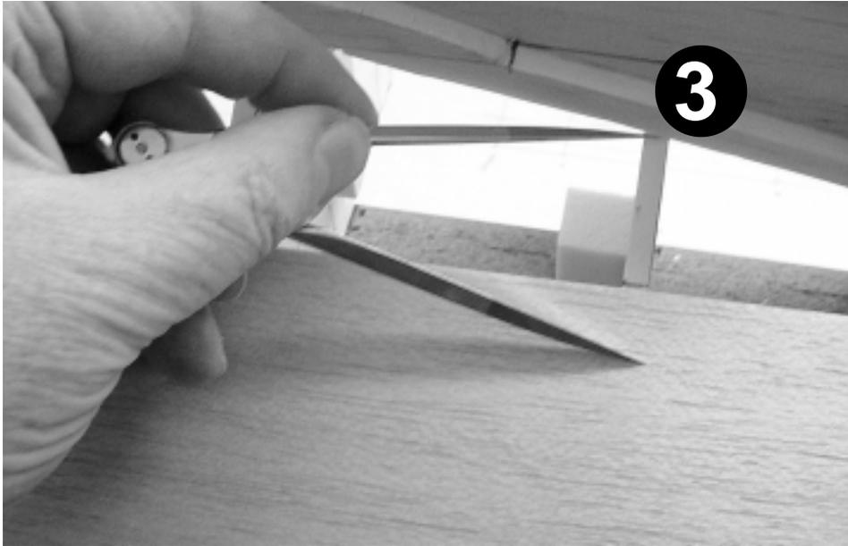
3. Now lay out and mark this distance from the keel onto the board at each station point. By doing this you are “sampling” the curve that must be put into the garboard plank for it to nestle tightly against the keel.
