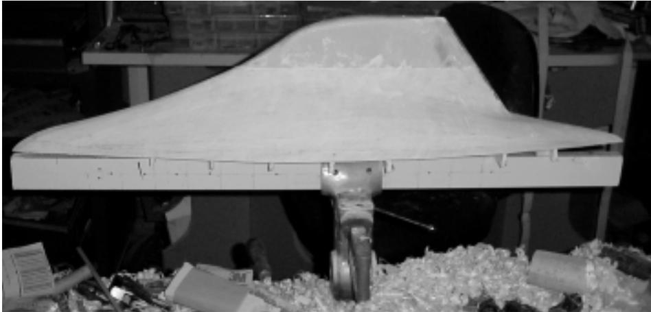
The hull has been roughly faired and covered with Micro-Fill in preparation for final fairing and glassing. The Micro-Fill will go on easier if you dampen the hull before rubbing it in. Wearing rubber gloves will shorten cleanup. Rub the filler into all the cracks, let harden well, then final fair with a *hard* block and 400 grit sandpaper. Long sweeping strokes, and as always sand diagonally and not directly fore and aft.
