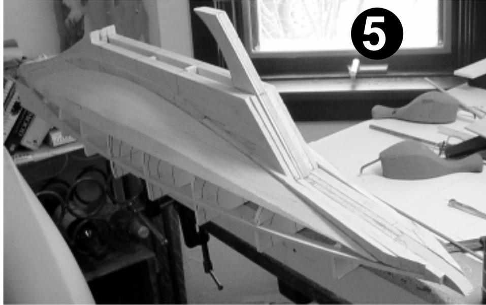
5. Subsequent layers, or “courses” of planks are done the same way: batten, distances, plot curve, cut and fit. This shows the second course. I got lazy and did the hull in three courses; it would have been better to have done it in four.
