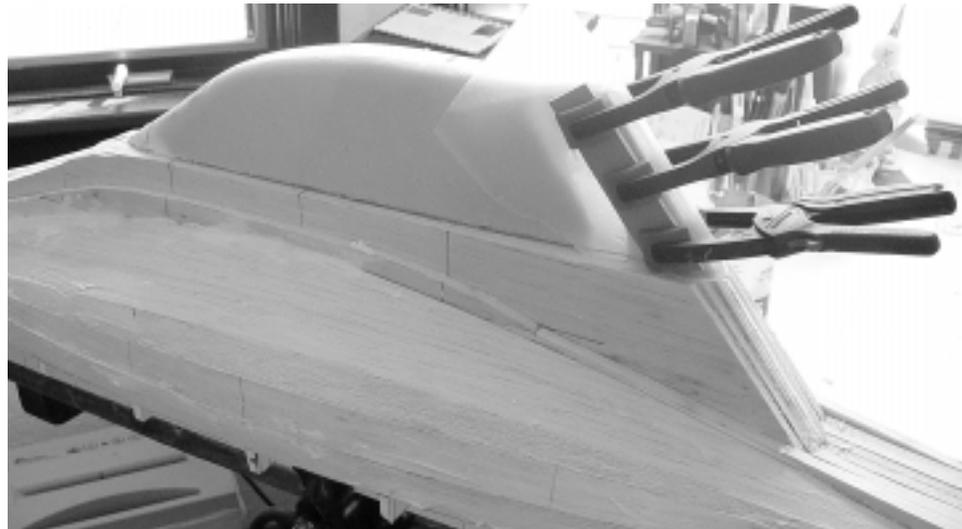
The fore and aft ends of the fin are hollowed out to fit the mounts on the hull. The fore mount is rounded to accept the shape of the fin, and the aft is tapered. The fin is then mounted to the hull with CA glue. This method makes it easy to align the fin properly.
