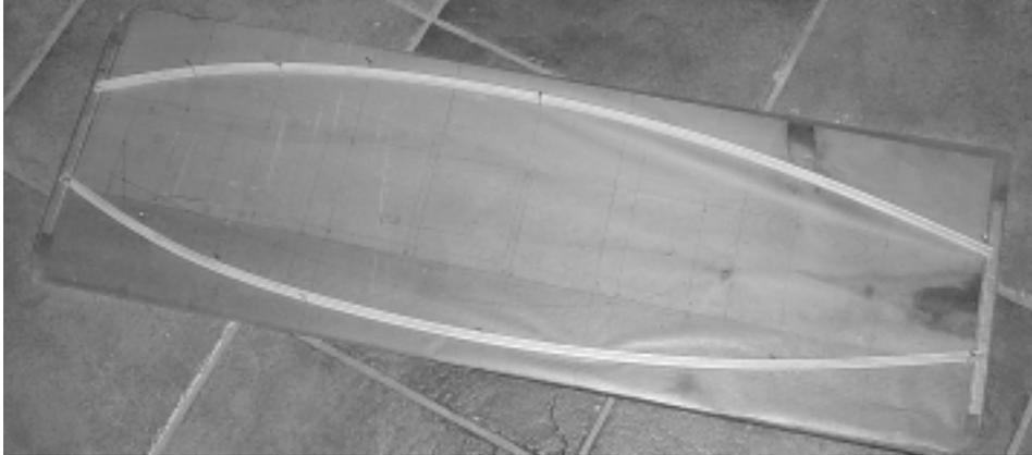
Make sure you lay out the strakes to the inside of the planking, as shown in the cross-section diagram.
